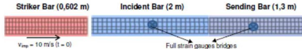
Fig.10. Mesh of the striker, incident and sending bars used for a Dynamic Finite Element Simulation of the SHPB device using Cast3M, Abaqus and LS-Dyna code
