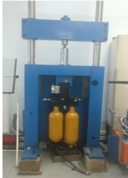
Fig. 9. Technological stand for the determination of the die geometry used in biomass pellet making equipment
