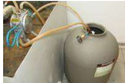
Fig. 13 - Recipient for the preparation of primary solutions; connections for suction- A_f / discharge- R_f of primary solution
