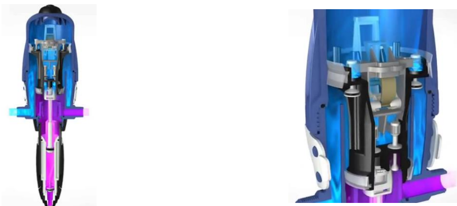
Fig. 7. Operation principle of the DOSATRON metering pump with differential piston
