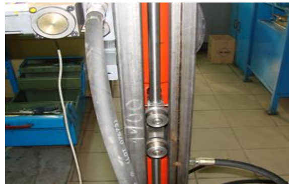
Fig. 5. Driveway slides detail, [2]
