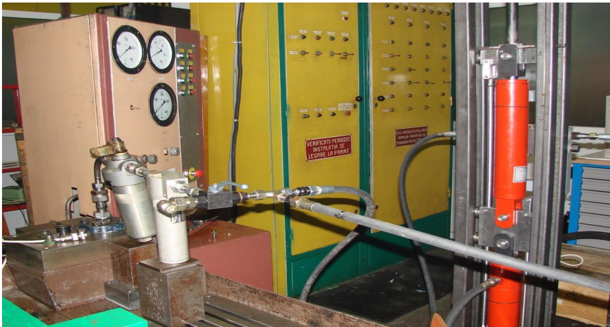
Fig. 6. Splitting the joint P of the stand in two cylinders power supplies,[2]
