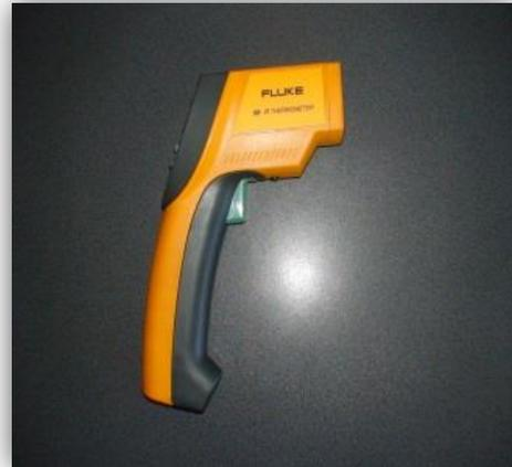
**Fig. 6.** FLUKE infrared thermometer
