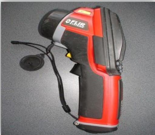
**Fig. 7.** FLIR infrared thermal imaging camera
