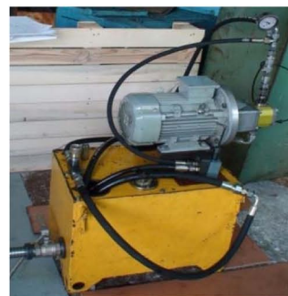
Figure 1. Test bench. a) Hydraulic scheme: HP-hydraulic pump; EM- asincron electric motor; C-coupling; T-tank; FAF-filling air filter; RF-return filter; V-valve; NRV non return valve; ST-suction throttle; RT-discharge throttle; G-pressure gauge; PRV-pressure limiting valve; FLUKE IT-infrared thermometer; FLIR IC- infrared thermal imaging camera; b) Picture of the test bench; c) Test bench thermogram.
