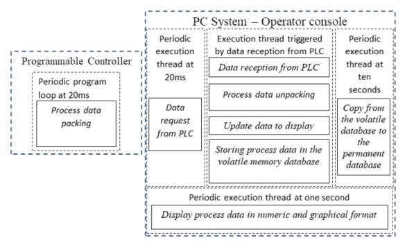
Fig. 2. Software architecture
