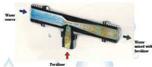
Figure 1. The operating principle of VENTURI type injector
