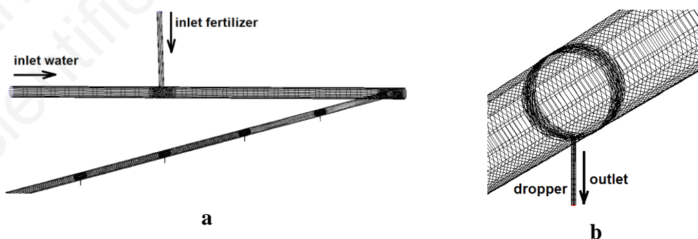
Fig. 3. Hybrid mesh model of the drip fertigation plants with droppers a. overview b. zoom in- dropper
