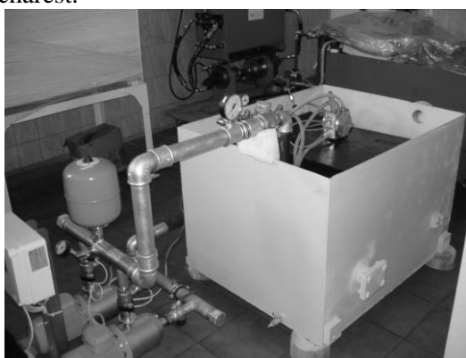
Figure 4 The hydraulic equipment tests stand using pressurized water as the working fluid
